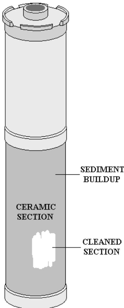
**If you are cleaning your ceramic cartridge at least six to eight times a year, you will find that installing a WaterRx Prefilter will keep you from having to clean your cartridge as frequently. The Prefilter will capture sediment that is 5 micron and above. The ceramic cartridge filters down to ½ micron. No form of bacteria can ever pass through the ceramic cartridge.**
