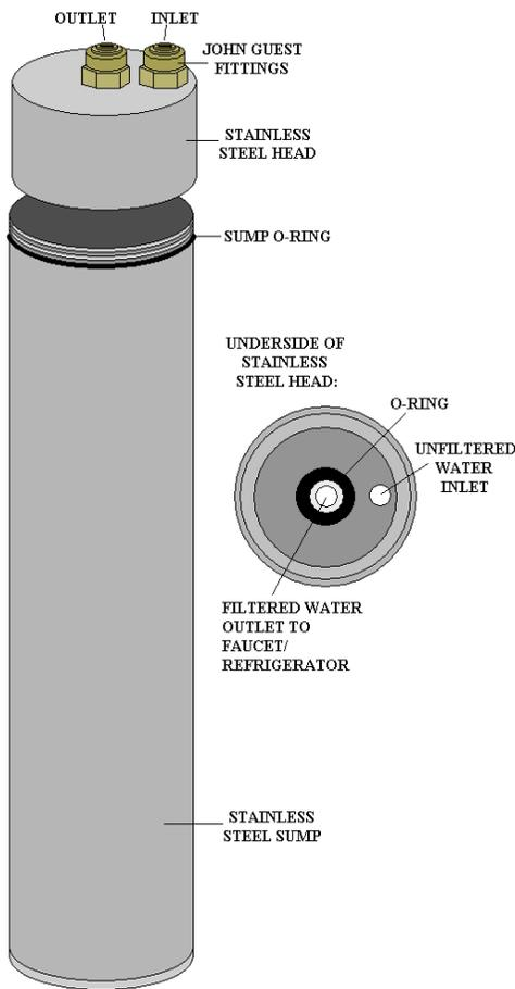
**When the rate of water flowing through your system slows significantly, it is time to clean the ceramic part of the cartridge only.**
